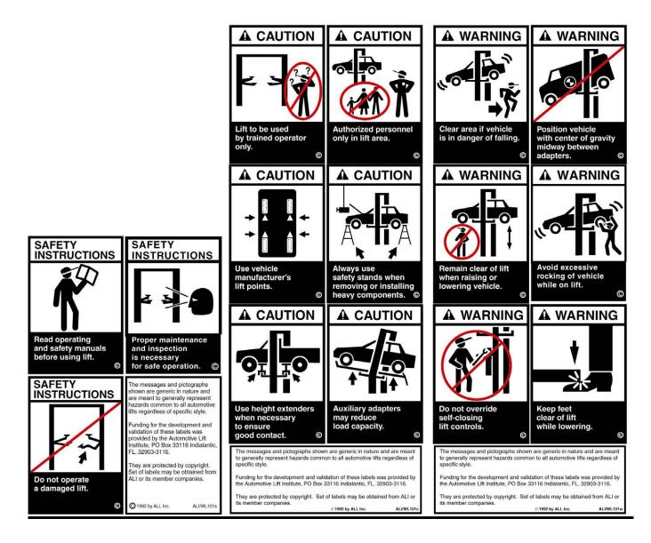
Ensure lift operators review safety and warning labels prior to operating lift.
