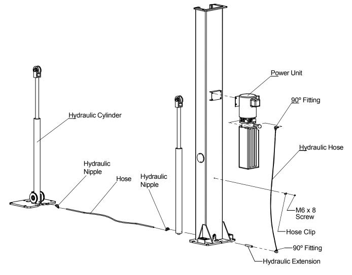
STEP 15: Mount the Power Unit on lift as shown.
