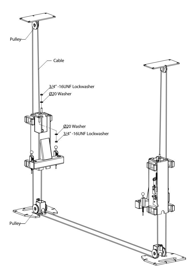
**STEP 13**: Cylinder centering and chain installation: Make sure the "Tip" on the bottom of the cylinder is properly located into the center hole on top of the cylinder mount in base. Pull the pre-attached leaf chain in both sides up and over the chain sheave on top of the cylinders.
