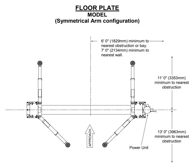
NOTE: Lift can be installed so power unit can column can be located on either side. However to save operation steps it is recommended that it is placed on passenger side of lift.
