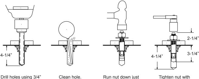
Drill holes using 3/4" carbide tipped masonary drill bit per ANSI standard B94.12.1977 Clean hole.
