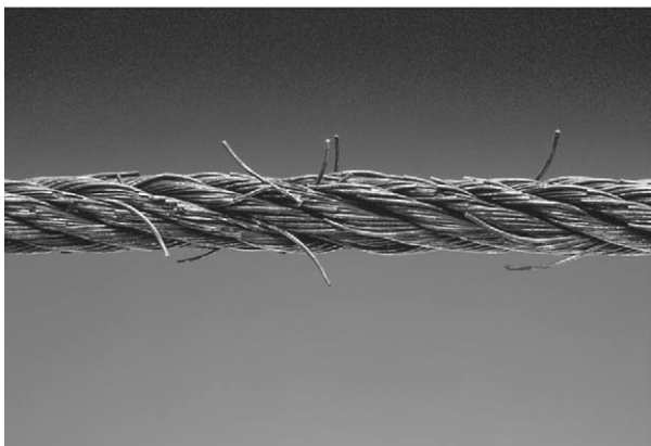
Cable With Severe Corrosion
