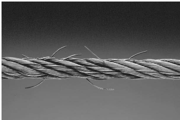
Cable With Broken Wires
