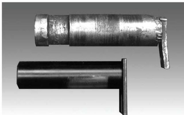
TOP PIN With Excessive Scoring and Wear
